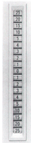
Fig. 9. Position of zero level baseline selected by Positioning control is indicated by illuminated numerals, enabling measurement of dc levels with analog voltmeter accuracy even with zero level displaced up to \pm 25 cm from center screen.
