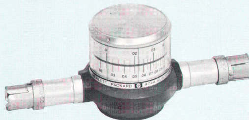
Fig. 2. -hp- Model 874A Calibrated Susceptance simplifies TDR measurements of small reactive discontinuities. Susceptance provides basis for comparison measurements of capacitive discontinuities from 0 to 1 pF and inductive discontinuities from 0 to 2.5 nH.
